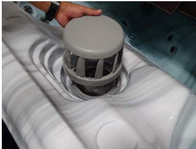
Figure 13. Weir cap removal
